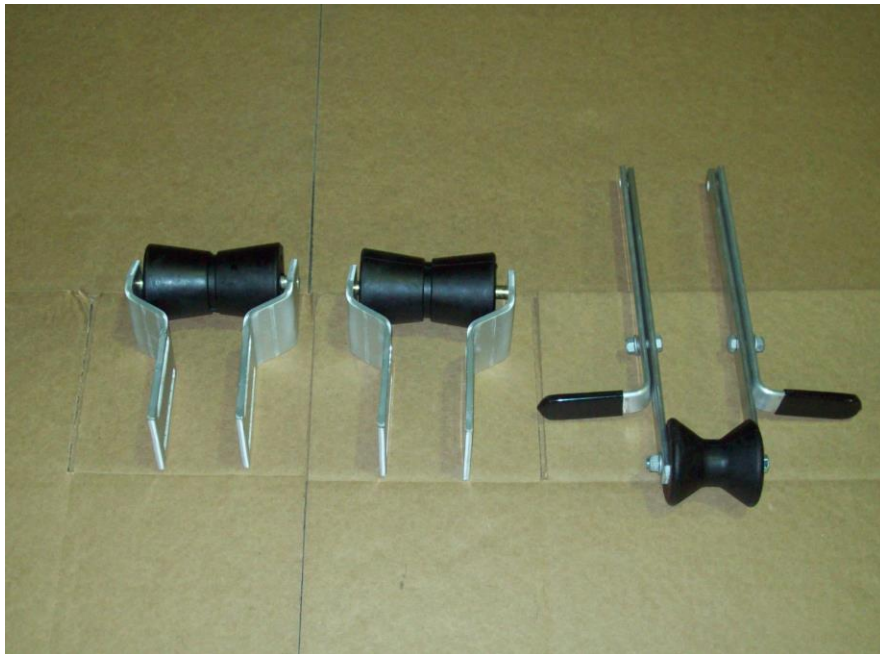
Rollers winch post and braces.
