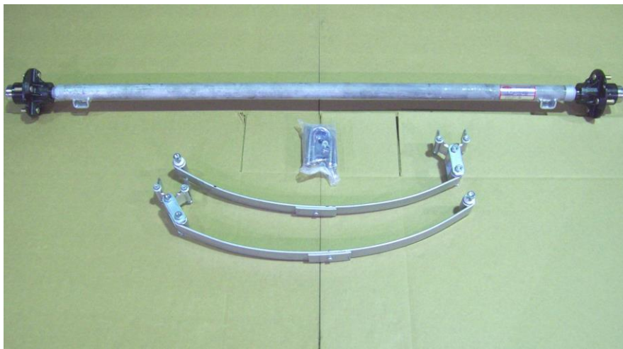
Axle assembly, springs and U bolt hardware.
